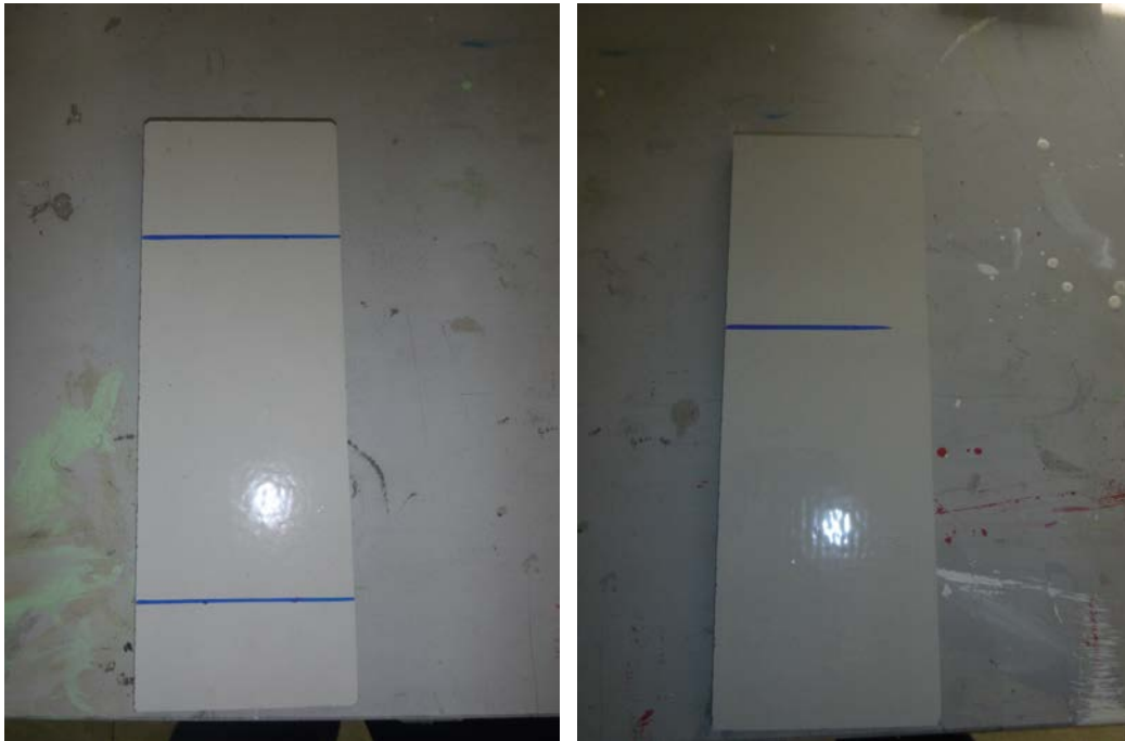
View of the sample before ignitability test according to EN ISO 11925-2: 2010 (application on edge)
